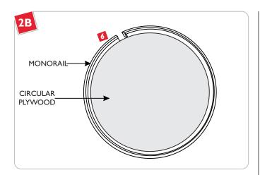
Start bending the rest of the Monorail against the circular plywood until the desired curve or circle is achieved.
