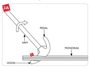
**NOTE:** The Wiremold Pipe Bender can be used to create smooth horizontal curve of 90° or less. Avoid stepping on the pedal of the Pipe Bender which will flatten and damage the Monorail.
