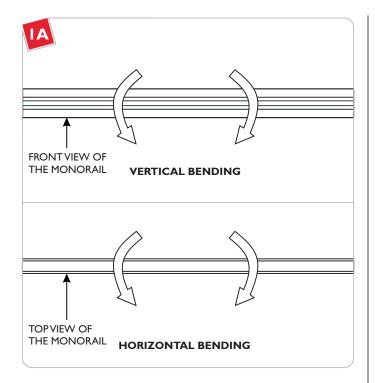
NOTE: There are three techniques for bending the Monorail horizontally, Plywood Template, Wiremold Pipe Bender, and Freestyle. When bending the Monorail vertically, only use the Wiremold Pipe Bender technique. Monorail bends horizontally easier than vertically. When bending the Monorail vertically, do small bends at a time and avoid bending the Monorail back which may cause the rails to separate from the insulator.
