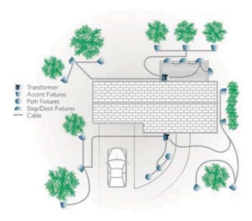
4. The correct **cable** needed for your job is determined by the length of the runs and the amount of wattage per run. Refer to the voltage formula on page 27 to assist you in selecting the proper gauge and length of cable. When laying out a job, always center feed to the group of fixtures on any single run. Avoid wiring to the closest fixture and continuing out from there in a straight line. Also, avoid heavily loading any single run. Keep run as short as possible.
